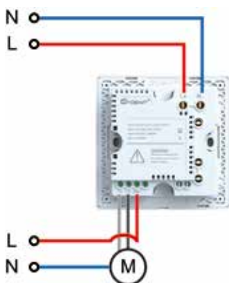
Connection 1: Dry contact (Strong electric)
